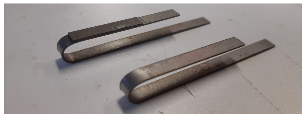
Figure 5.3: U-shaped iron body with and without glued Galfenol sheet.
