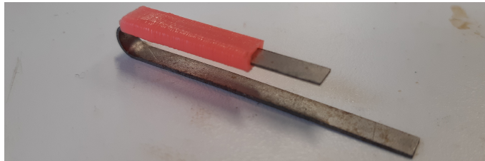
Figure 5.4: U-shaped body with Galfenol sheet and 3D-printed wiring piece.
