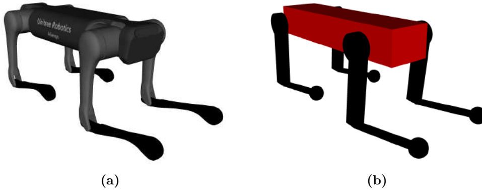
Figure 4.2. AlienGo quadruped URDF model: (a) Geometric model, (b) Collisions model.
