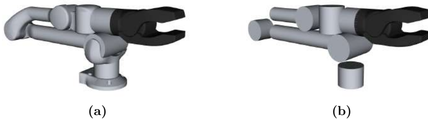
Figure 4.3. Z1 manipulator URDF model: (a) Geometric model, (b) Collisions model.
