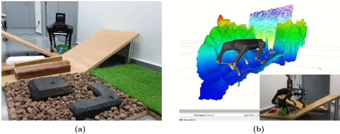
Figure 5.24. Unitree A1 quadruped NMPC controller testing [129]: (a) Obstacle track, (b) Elevation map generation.
