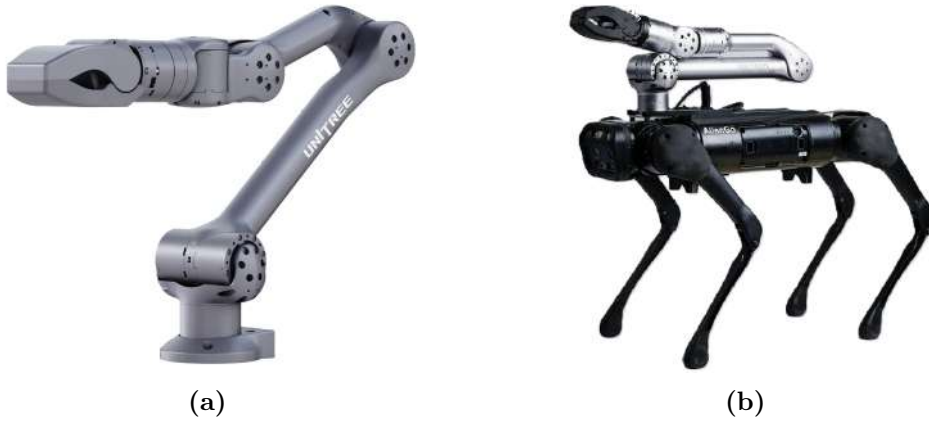
Figure 3.3. Integration of Unitree AlienGo quadruped and Z1 manipulator [86]: (a) Unitree Z1 manipulator, (b) Z1 manipulator mounted on AlienGo quadruped.
