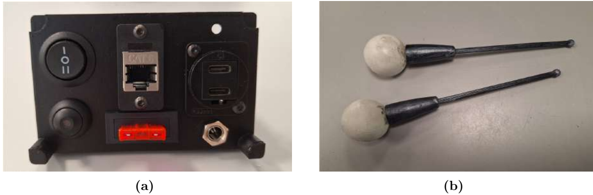
Figure 5.5. 3D-printed parts: (a) Ports panel, (b) Antennas.
