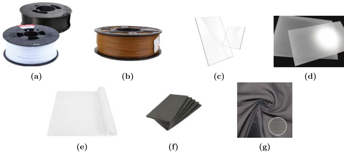
Figure 5.1. Robot materials selection from RS Iberia and Amazon: (a) PETG 1.75 mm filament, (b) ABS 1.75 mm filament, (c) 2 mm transparent PVC panel, (d) 3 mm polystyrene panel, (e) 3 mm silicone sheet, (f) Anti-slip foam adhesives, (g) Nylon elastic textile mesh.
