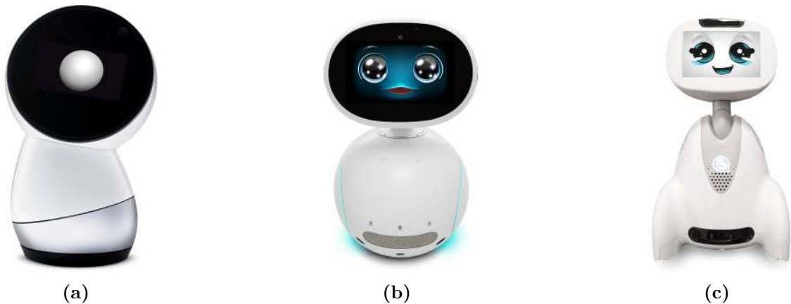
Figure 2.6. Examples of social robots used for personal assistance: (a) Jibo [51], (b) Zenbo [52], and (c) Buddy [53].
