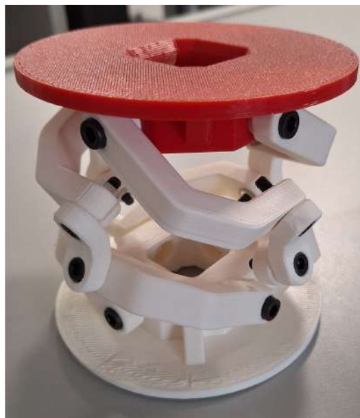
Figure 4.23. Testing initial neck mechanism prototype.
