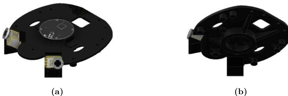
Figure 4.14. Details of the head structural support: (a) Top view, (b) Bottom view.
