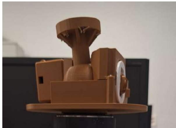
Figure 7.2. Detail of the top cover of the spherical gear mechanism.
