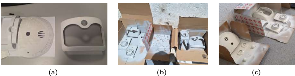
Figure 5.4. Post-processing steps: (a) Putty application on the front and top head panels, (b) Priming process, (c) Painting process.
