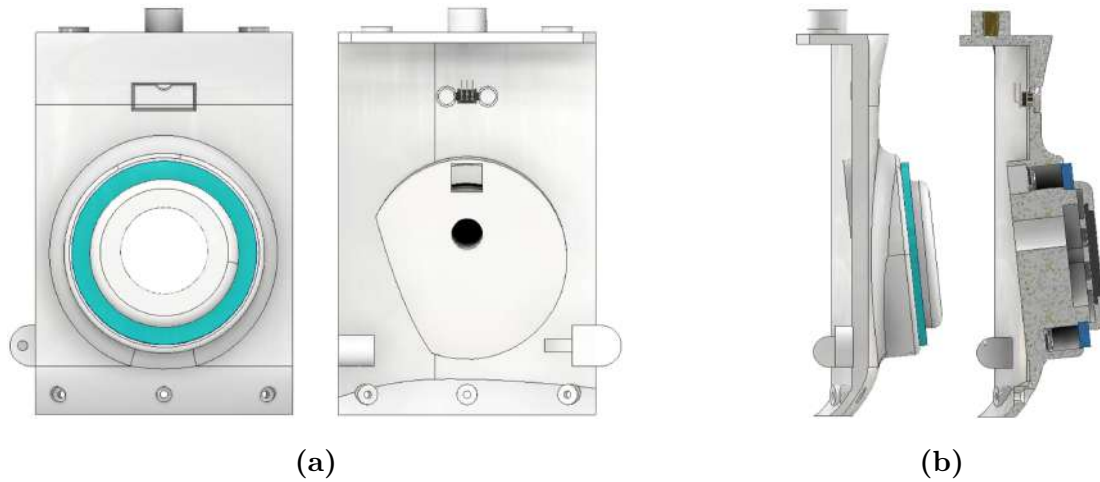
Figure 4.16. Details of the head lateral panels: (a) Front and back views, (b) Side view and cut view.
